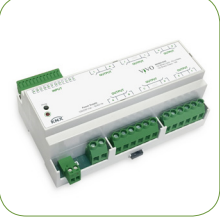
NANNA KNX Product Code: K.NAN.01O.20N.WO 12x Binary Input - dry contacts and 12x Binary Output - 16A / Ingresso binario 12x - contatto pulito e Uscita binaria 12x - 16A
